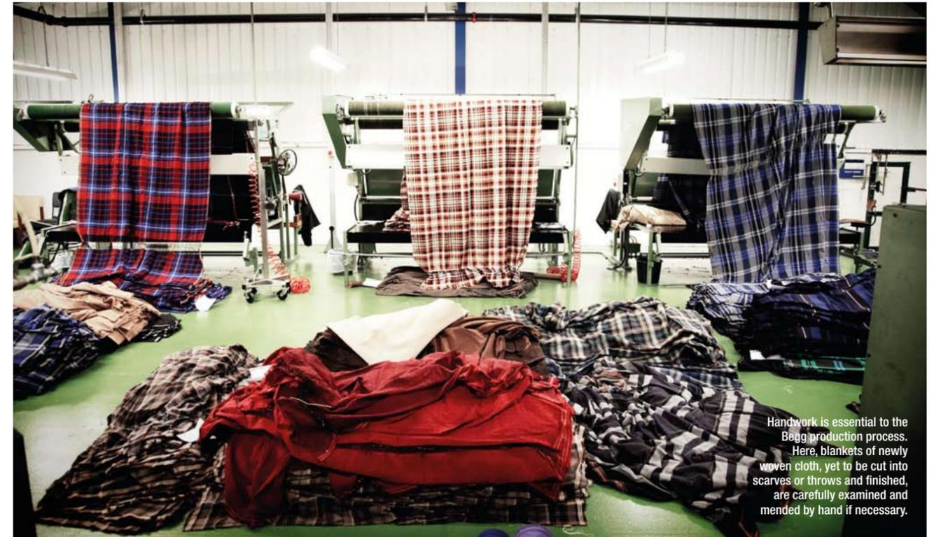
Handwork is essential to the Begg production process. Here, blankets of newly woven cloth, yet to be cut into scarves or throws and finished, are carefully examined and mended by hand if necessary.
